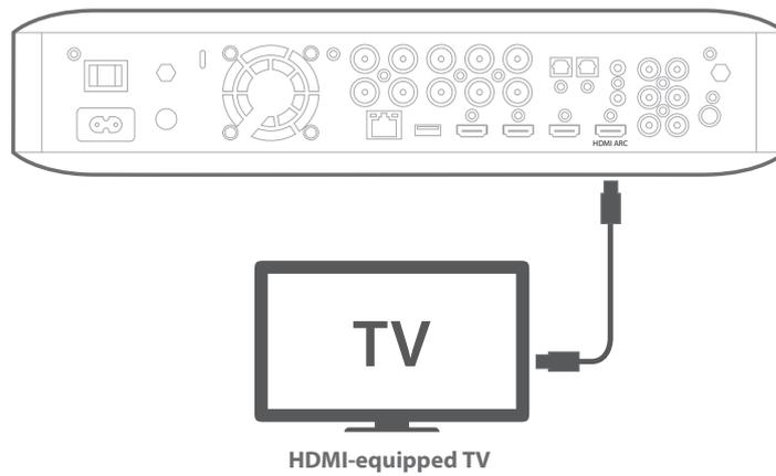
**NOTE:** If your TV supports HDMI Audio Return Channel (ARC) and you access digital channels from your TV's built-in tuner or you have other sources (such as a component video source) already connected directly to your TV, you can feed their sound to the BDS system via the HDMI Monitor Out connector's Audio Return Channel, and they will not require additional connections to the system.
