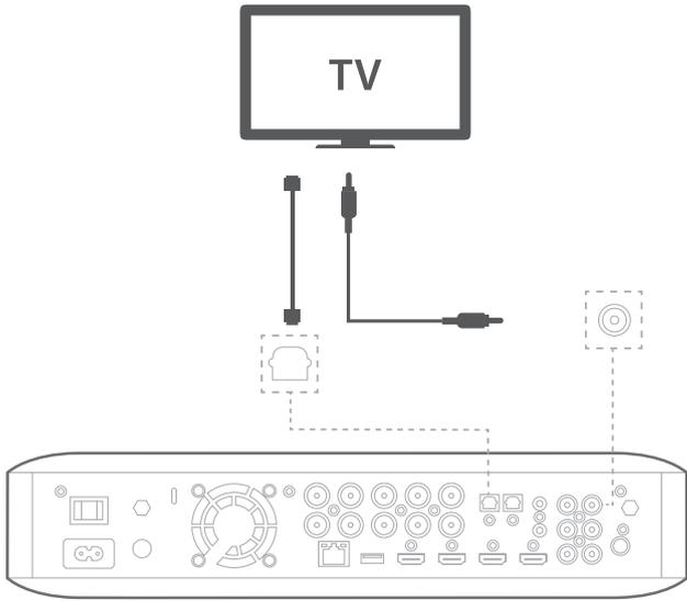
Connecting an analog audio source device
