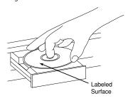
To retract the drawer back into the player after loading a disc, press the **Open/Close** button **3** . When the drawer is closed the display will indicate the total number of tracks on the disc and the total running time of the disc.
